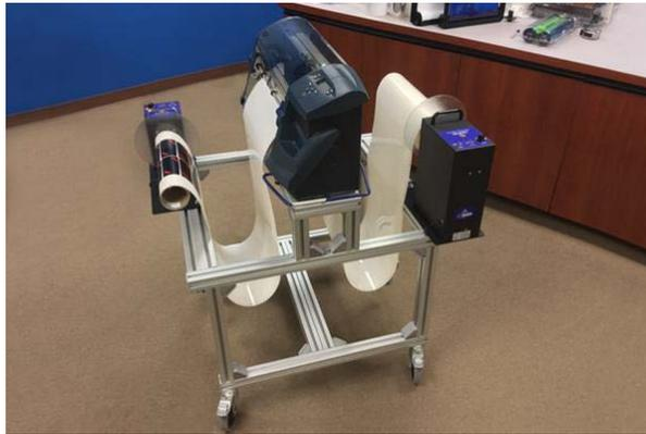
Both printer and cutter with their own unwinds/rewinds, can operate unattended, except for ribbon or roll changes.
