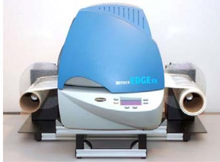
*Gerber Edge FX on GMS Alignment frame with unwind/rewinder*
